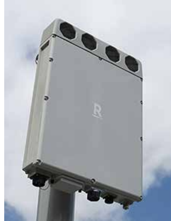
NEC built this 5G Open RAN radio unit for use by Rakuten Mobile.
