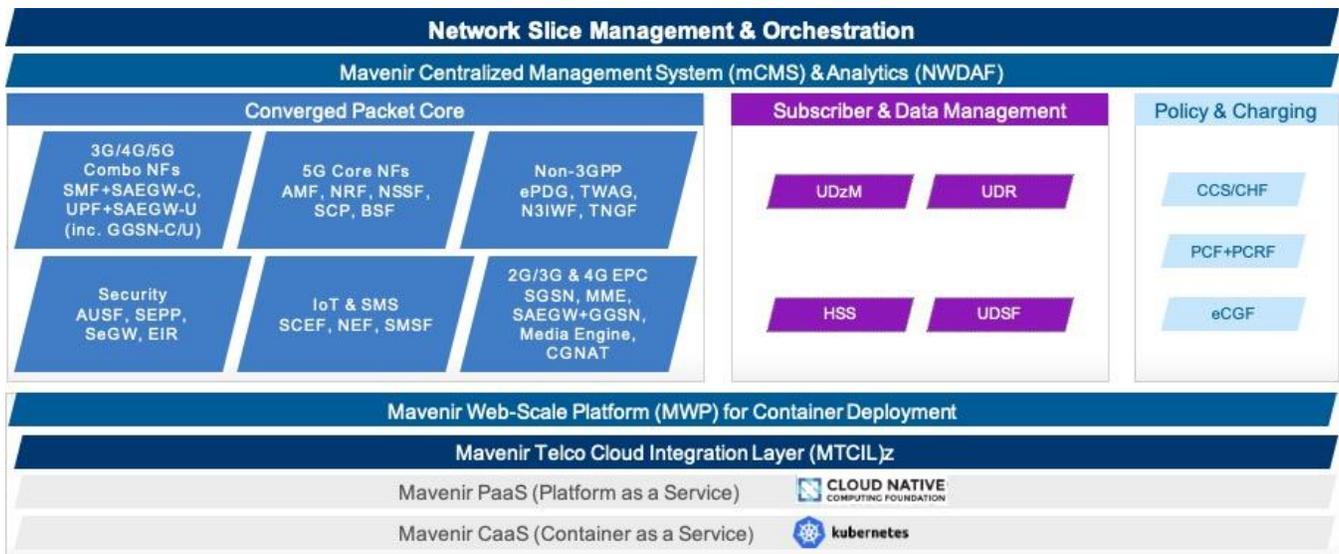
Figure 1: Mavenir Converged Packet Core Solution Components
